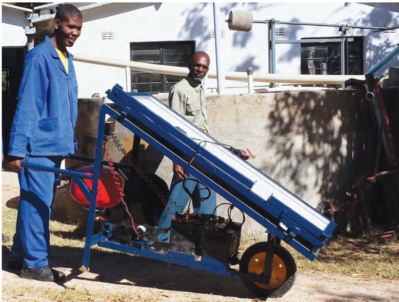
Using sustainable solar power to operate simple pumps to raise water. Photo: QSA
